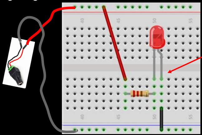
If the LED does not Light, Pull it out and turn it around to "Flip" the Pins
