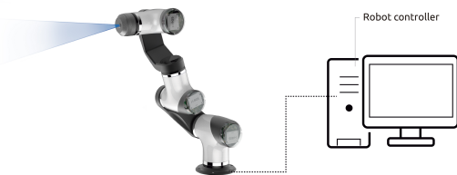
Fig. 1: Experimental setup with a 6 Degrees-of-Freedom (DoF) modular articulated arm and a range finder
